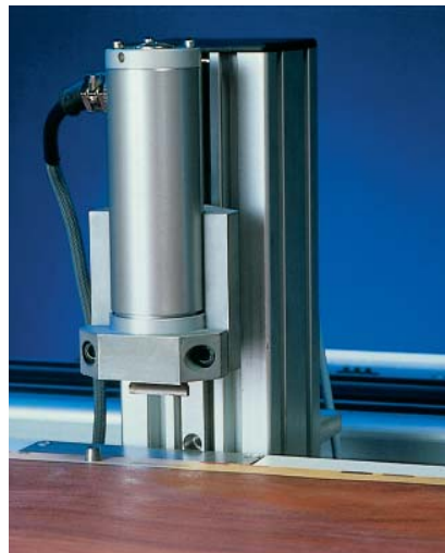
Ultrasonic track - welding
