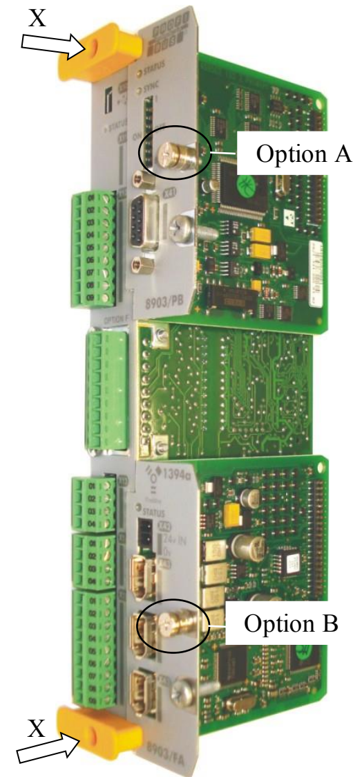
Figure 2 Control board with an Option Card correctly mounted
